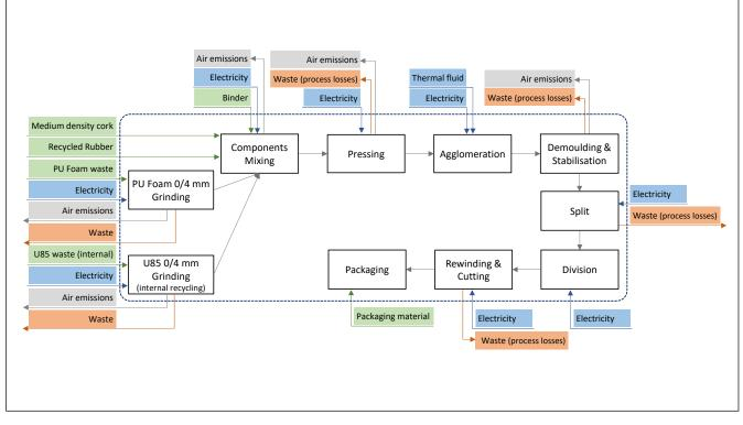
The Underscreed U85 production comprises 11 stages: Medium density Cork Grinding (outside ACC facilities), PU Foam 0/4 mm Grinding, U85 0/4 mm Grinding (internal recycling), Components Mixing, Pressing, Agglomeration, Demoulding & Stabilisation, Split, Division, Rewinding & Cutting and Packaging.
